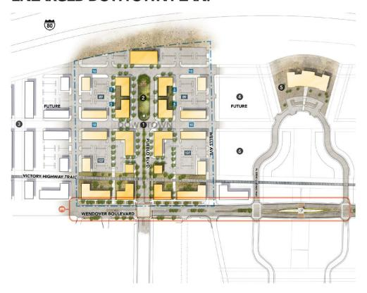
This enlarged view of the downtown master plan shows the first phase with suggested building footprints and parking layouts as well as the Festival Plaza configuration. The grid established by the first phase becomes the ordering principle for the expansion to the west and the transition space between the new downtown and the Civic Center.
